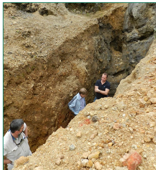
Quetzal Project: High-grade Zinc-lead-silver exposed in surface trenches
